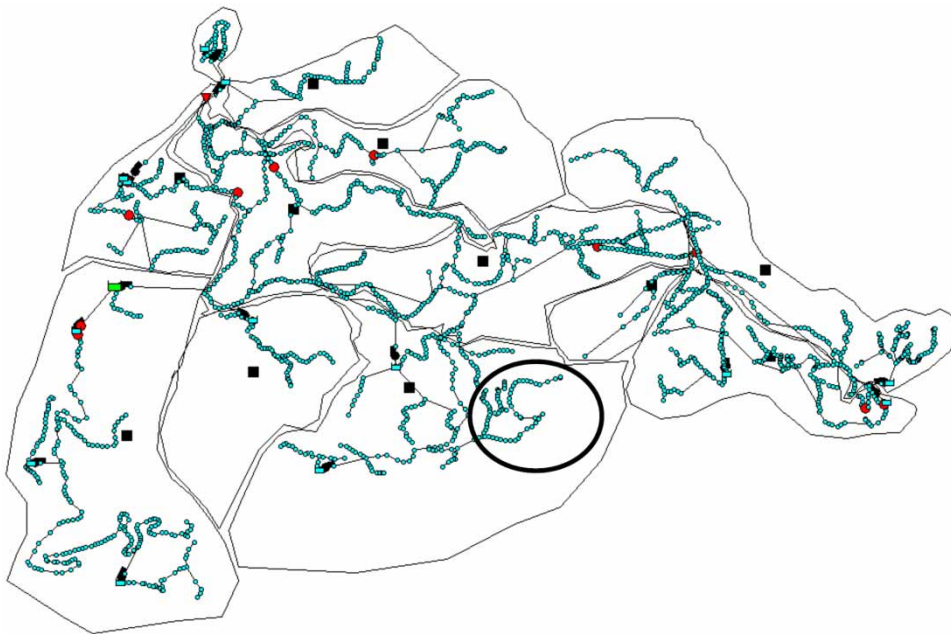
Figure 3 | Massa Lubrense network; the area with a double probability that it is the source of contamination is indicated by a circle. The dots represent the current location of 12 existing sensors that are used to calibrate the model.
