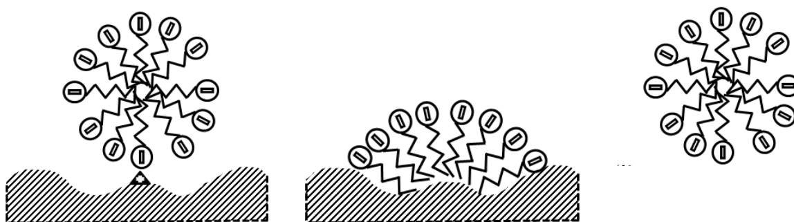
Figure 2.8 Illustration demonstrating the formation of micellar structures. A) Formation of a micelle from aggregated PFAS, attached to a surface functional group by charge. B) Formation of surface hemi-micelle - by either surface charge or hydrophobic interactions resulting in sufficient aggregation. C) Free floating micelle in solution where PFAS concentration is above critical micelle concentration.
