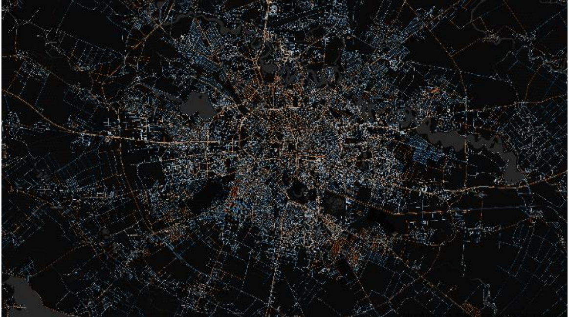
Figure 8. Plot of the Bucharest OSM graph where segments are color coded based on the length.
