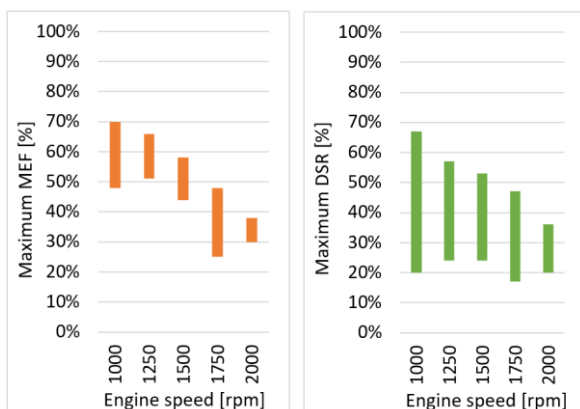
Figure 7: Ranges for maximum MEF and DSR as a function of engine speed.
