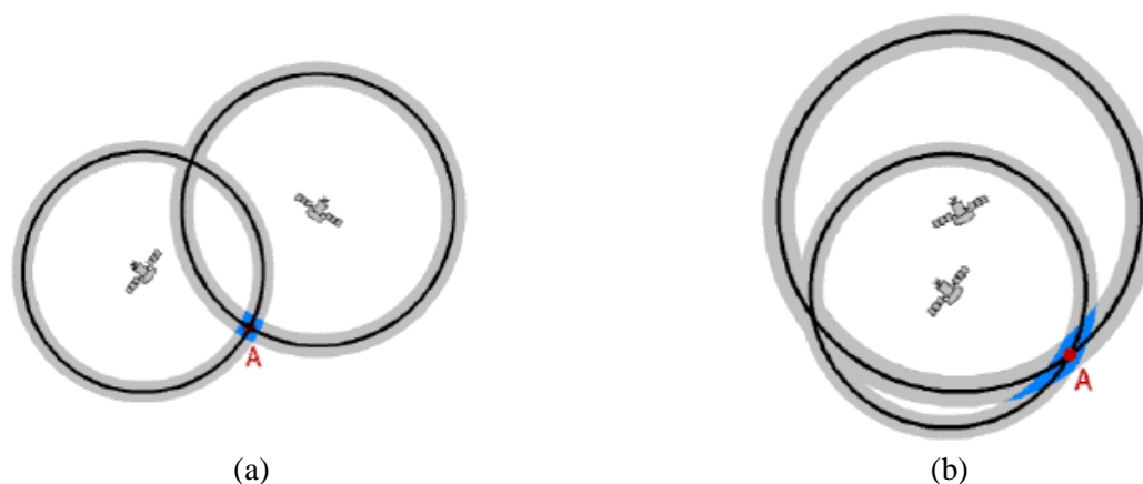
Fig. 1 (a) Good satellite geometry, (b) Bad satellite geometry
