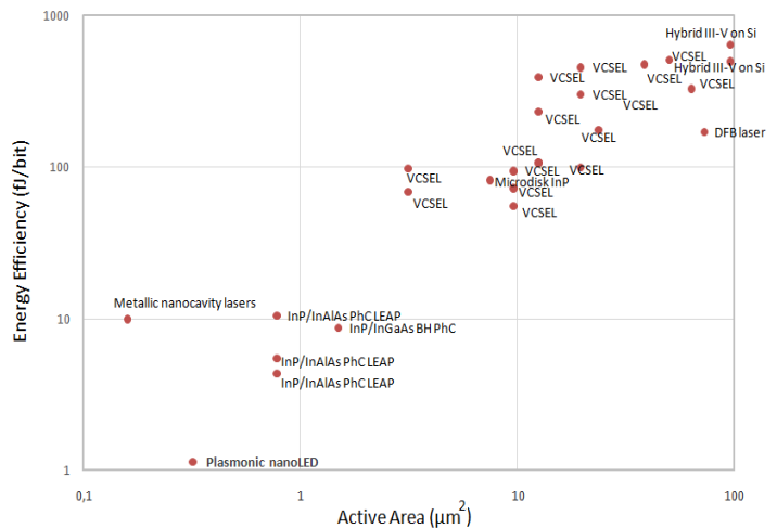
Fig. 16. Active area vs energy efficiency for directly modulated sources (data from Table 4)
