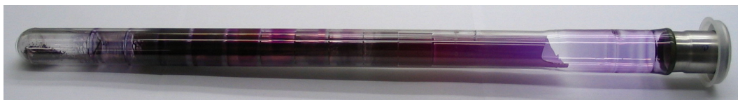
Figure 3.3.: Picture of a sublimation tube after sublimation. On the left end of the tube, remainders of the original material are visible. The image was taken by Annette Petrich.
