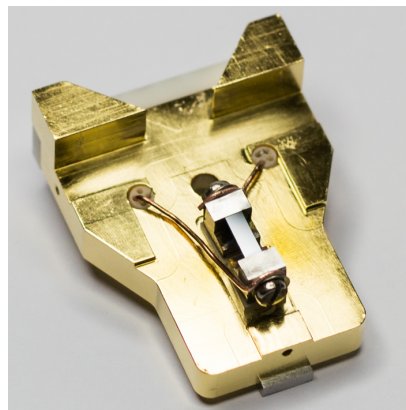
Figure 6.4 – Silicon sample holder with mounted Si(100) sample.
