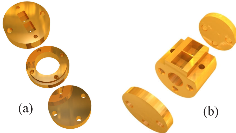
Figure 3.12: Axial (a) and transverse (b) resonant cavity. Two axial cavities (W3a, W4a) were constructed for W-band. Different resonance frequencies are achieved by exchanging the cylindrical body with one of different dimensions. In total four transverse resonators were built. Two resonators at V-band (V1t, V2t) have the same dimensions, but V2t has 0.2 mm wide cuts at 1/4 and 3/4 of the length of the cylindrical body. The transverse resonators at W-band (W1t, W2t) have different inner diameters and with that different resonance frequencies (cf. Table 3.2)
