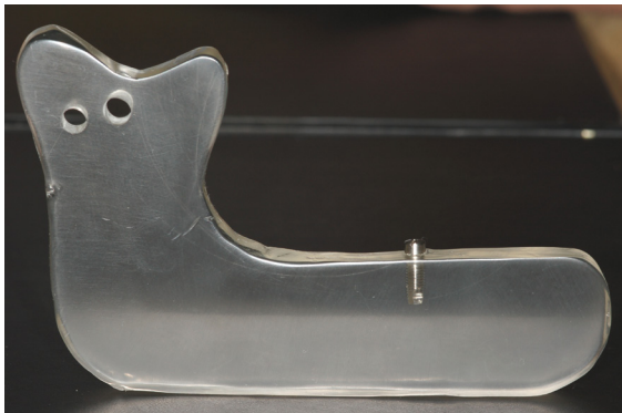
Figure 3 - Prepared photoelasticity model
