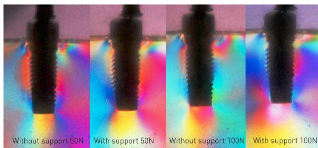
Figure 6 - Chromatic changes around the implants at different loads with and without support
