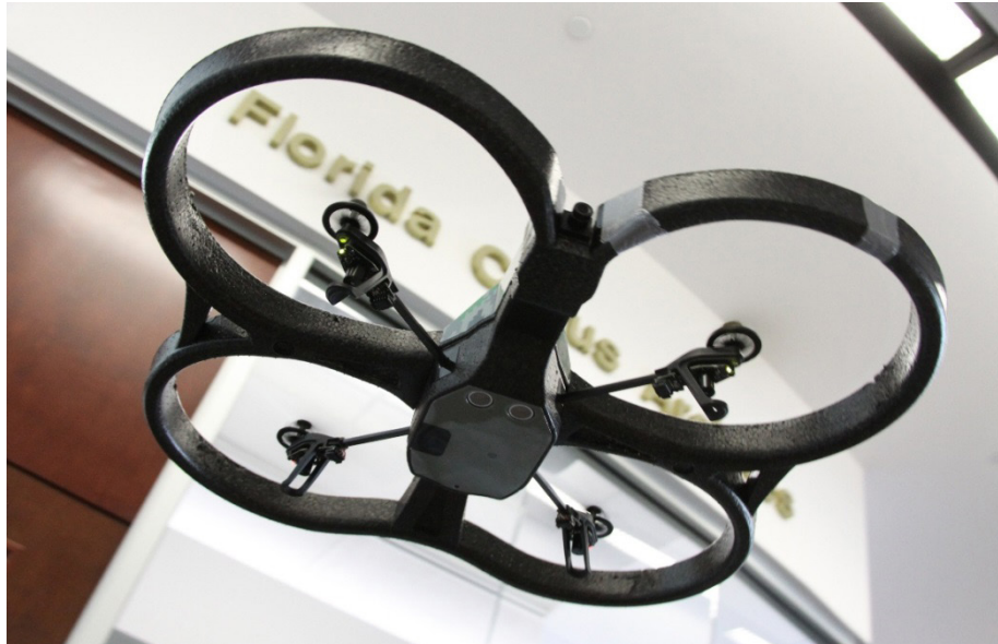
Figure 2: The A.R.Drone 2.0 in flight. The front-facing camera, bottom-facing camera and ultrasound sensors.
