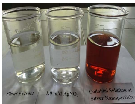
Figure 1. Photograph of (A) Cucurbita lagenaria L. fruit extract, (B) 1.0 mM AgNO 3 solution without fruit extract, (C) Colloidal solution of silver nanoparticles
