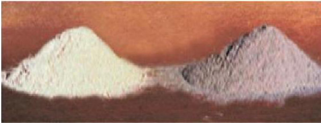
Fig 4. Typical ash colors (Class „F“ & „C“ Fly ash) (Source:- International journal of emerging trends in Engineering and Development Issue1, Vol 1August2011)
