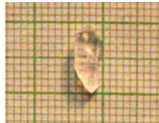
Fig.1. As-grown single crystals of LAA
