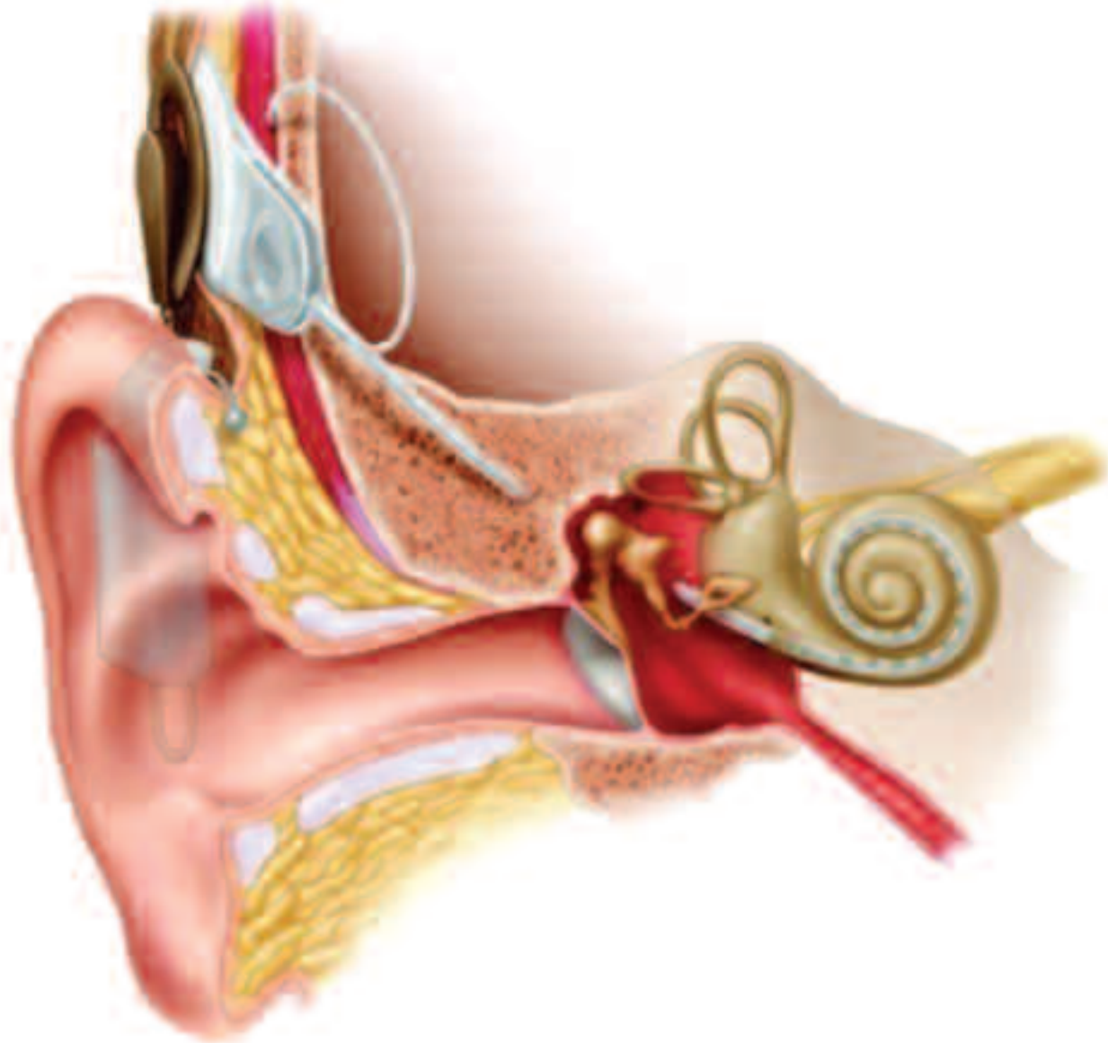
FIGURE 2 | Cochlear implant internal components: receiver stimulator under the scalp and electrode array passing through the mastoid bone into the cochlea (courtesy of Cochlear Limited).
