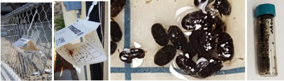
Fig. 2 Storgard II sticky trap hung on a fence near the periphery of a research site (left). Beetles fly to the red rubber stopper that is slowly releasing the synthetic female sex pheromone, and then are stuck on the sticky trapping surface inside the trap (second from left). Adult Trogoderma are found in the trap (second from right), removed and cleaned in solvent prior to being identified to species and counted (right).
