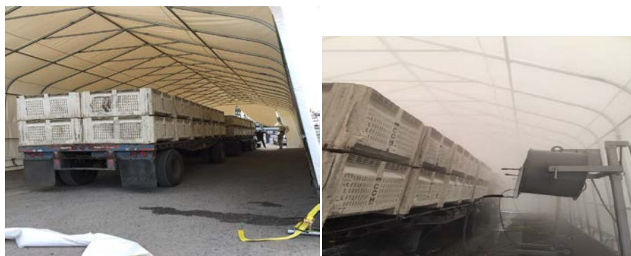
Fig. 6 The high-pressure fogging with an aqueous mixture containing 0.1% Evergreen® (6% pyrethrins & 60% piperonyl butoxide) and 0.5% (v/v) BreakThru® (polysiloxane surfactant) can be conducted on a 48-bin trailer load driven into a tent structure, methodology that is consistent with the need to disinfest field-run fruit prior to its exiting the grove.
