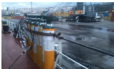
Fig. 2 Eight ECO2FUME® cylinders secured and connected in manifold during gas dispensing through the hatch.
