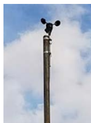
Fig. 2 HOBO Wind Speed Smart Sensor attached to top of pole to measure wind speed free from obstruction
