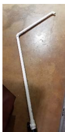
Fig. 1 Extension arm created from PVC pipe to extend down side of bin for pressurization using shop vacuum
