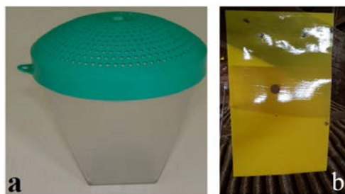
Fig. 1 Cone trap used for monitoring of Habrobracon hebetor (a) and adhesive trap baited with sex pheromone (ZE-TDA) (b) for monitoring of Plodia interpunctella in flat grain storage.
