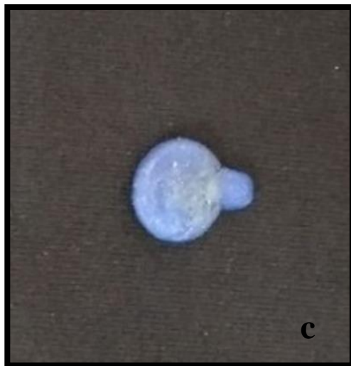
Fig. 34c: Light cured millable resin disc
