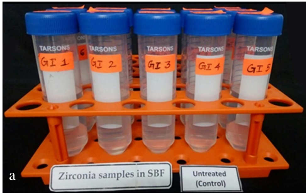
Fig. 50a: Group I (Untreated) test samples in SBF (n=10)
