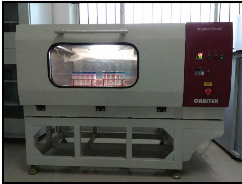
Fig. 53: Incubation of test samples at 36.5°C
