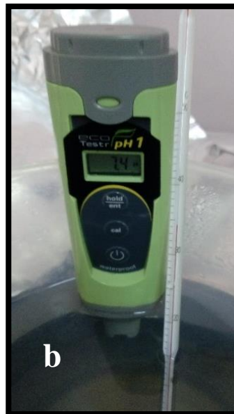
Fig. 47b: pH tester showing pH 7.4 for the SBF solution
