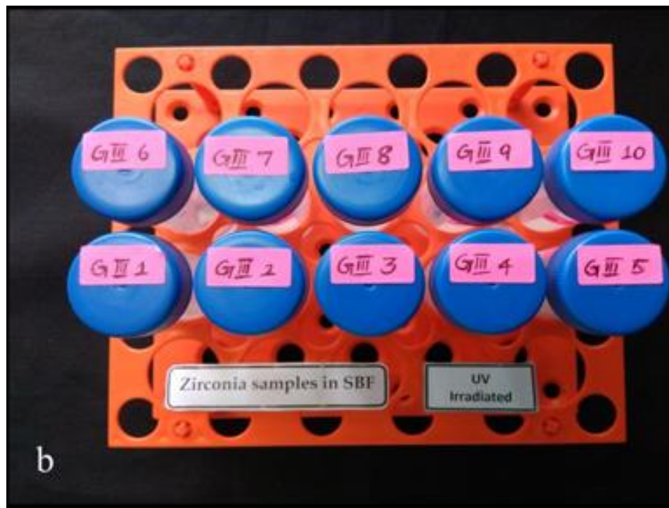
Fig. 52a: Group III (UVP) test samples in SBF (n=10)
