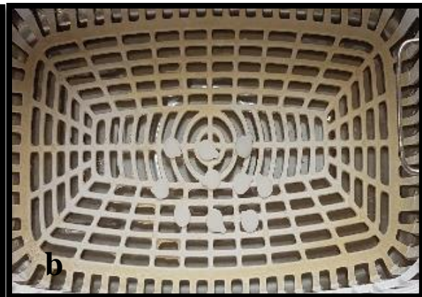
Fig. 39b: Samples placed in the ultrasonic bath
