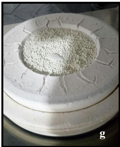
Fig. 34g: Zirconia sample after sintering at 1500°C for 8 hours
