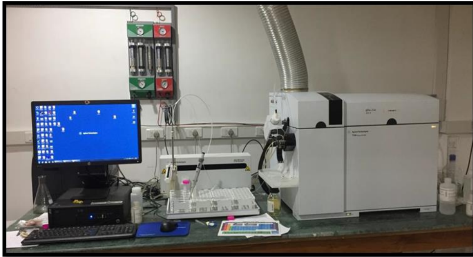
Fig. 55: Analysis of calcium content in SBF using ICP-MS
