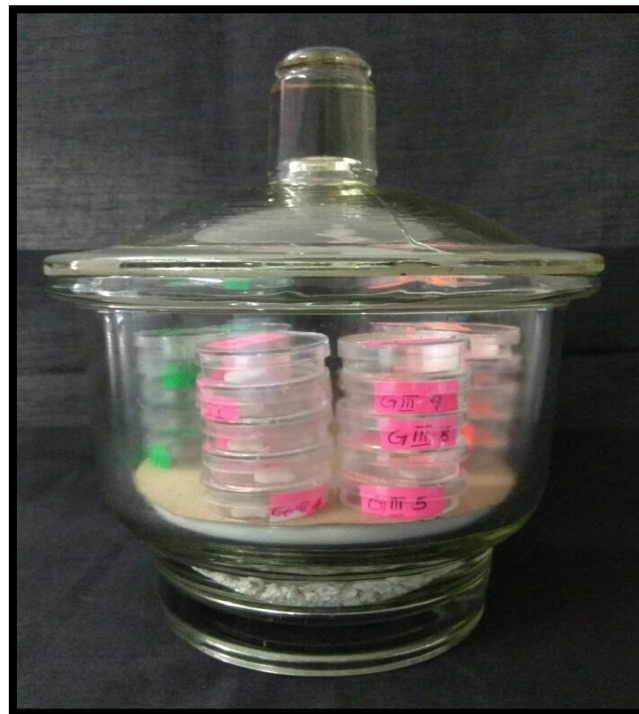
Fig. 42: Test samples of Groups I, II & III stored in Desiccator for further analysis
