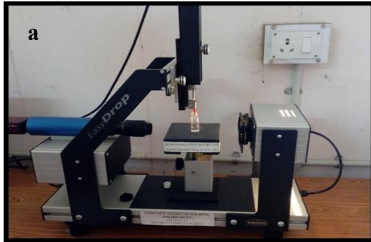
Fig. 45a: One \mu\text{l} of water placed on platform for contact angle measurement
