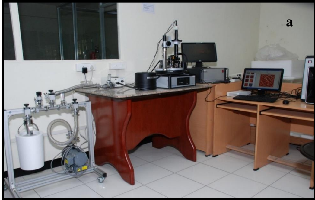
Fig. 26a: Set –up for Multimode Scanning Probe Microscopy (Atomic Force Microscopy) unit
