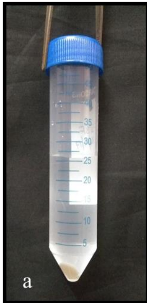
Fig. 49a: Immersion of a test sample in SBF solution in a graduated test tube
