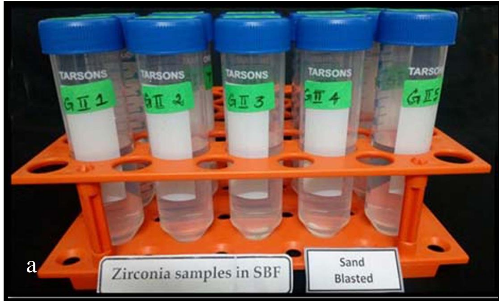
Fig. 51a: Group II (Sandblasted) test samples in SBF (n=10)
