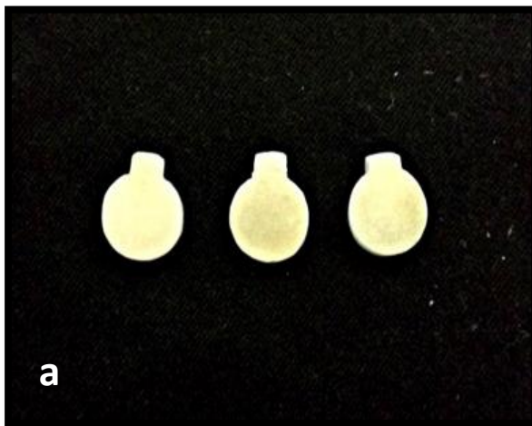
Fig. 46a. Gold sputtered test samples of Groups I, II and III for SEM – EDX analysis
