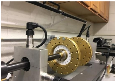
Figure 5. 1 Unbalanced fault simulation
