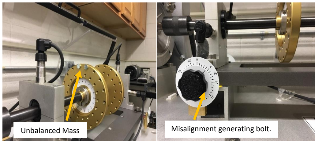
Figure 2. 4 Unbalanced and misaligned condition simulation.
