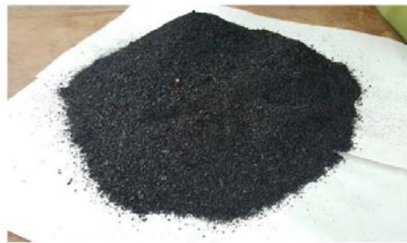
Figure 1: Saw Dust Ash (SDA)
