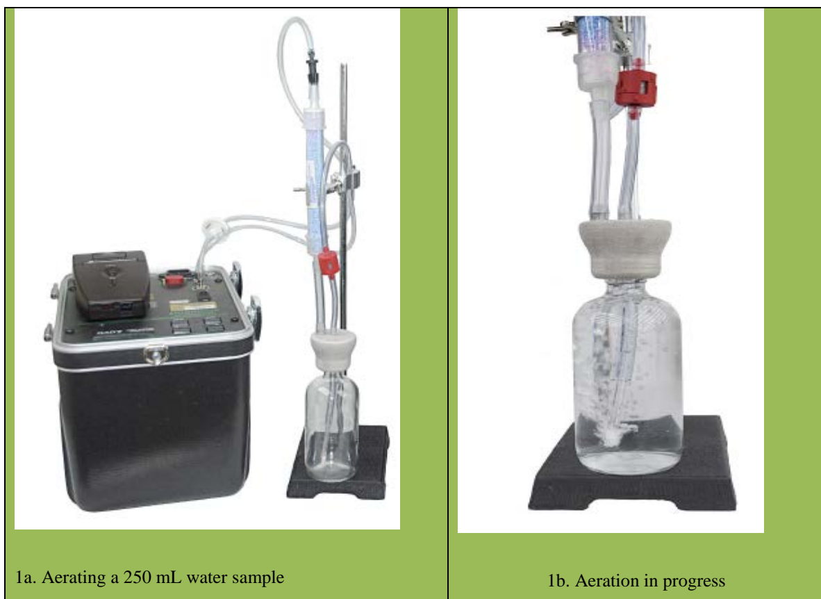
Figure 1: Measurement apparatus RAD 7 (RAD H 2 O User Manual)
