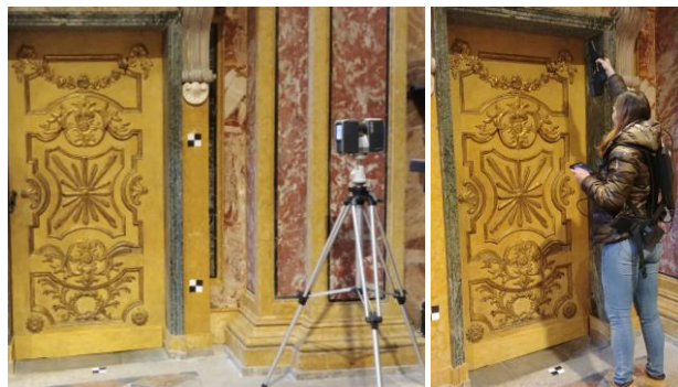
Figure 7a and b. TLS and F6 SMART data acquisition.
