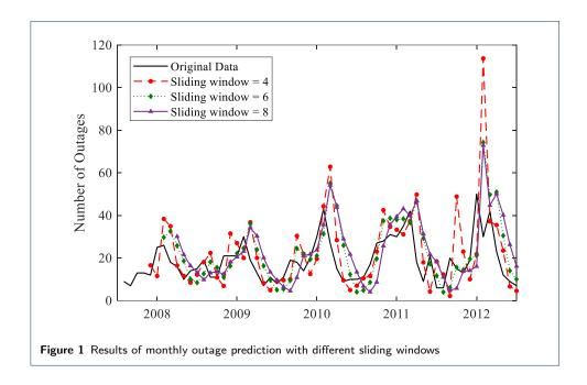
for a stronger power grid. The parameters for building the traditional grey model GM(1,1) is first improved with the optimization techniques. Since the monthly outage number is a seasonal data sequence, the rolling mechanism is introduced to improved the ability of capturing the change of trend.
