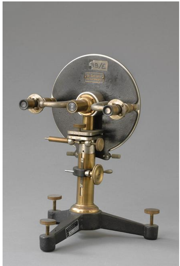
Fig. 6. Two Field Lippich Twilight Analyzer. A device used for the determination of straight-line polarized light when it crosses a certain thickness of optically active substances.
