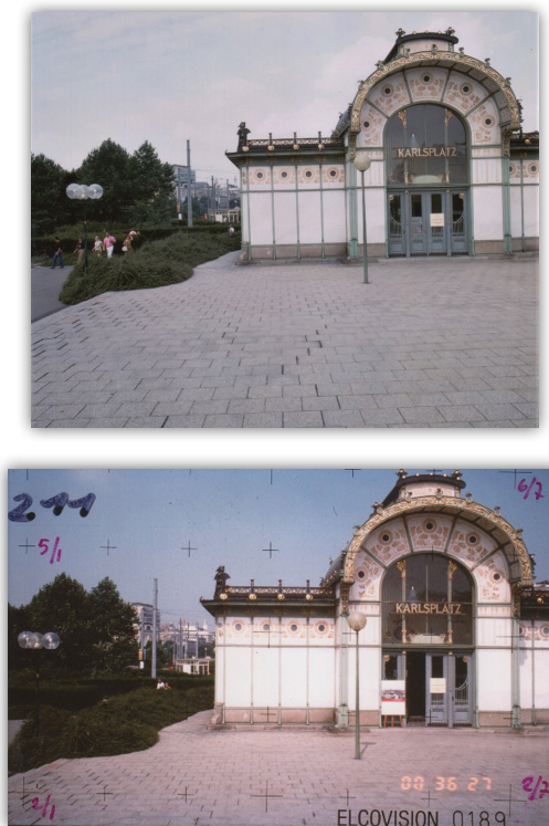
Figure 1. Semi-metric and amateur images: amateur Hasselblad camera (up), semi-metric LEICA Elcovision camera (down).
