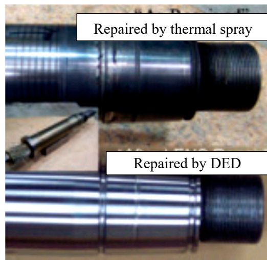
Figure 11. A drive shaft repaired by thermal spray (top) and DED (bottom) processes [87].
