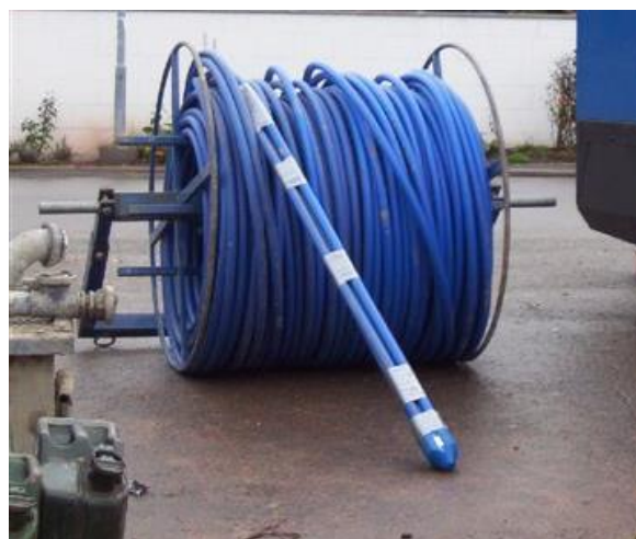
Figure 1. Example of vertical ground loop heat exchangers made by high-density polyethylene U-tube pipes; common diameters range from 19 mm to 38 mm.
