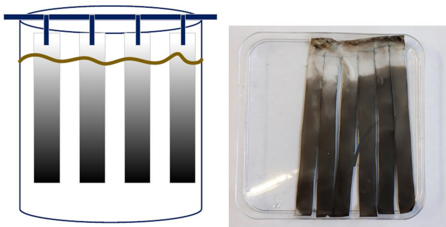
Figure 7.1: PDA-coating set-up for electrospun TPU fibres; the scheme of the set-up is shown on the left and the actual final product (TPU-PDA-LPO-1.4-7) is shown on the right.
