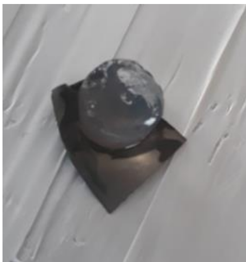
Figure 8.3: TPU-PDA-GO-1.4-7 (1 cm x 1 cm) with 100 \mu L glucose-loaded GelMA hydrogel.
