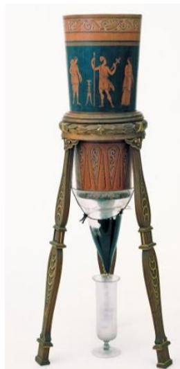
Figure 1: The condensation-based hygrometer exploited by Ferdinand-II [9]
