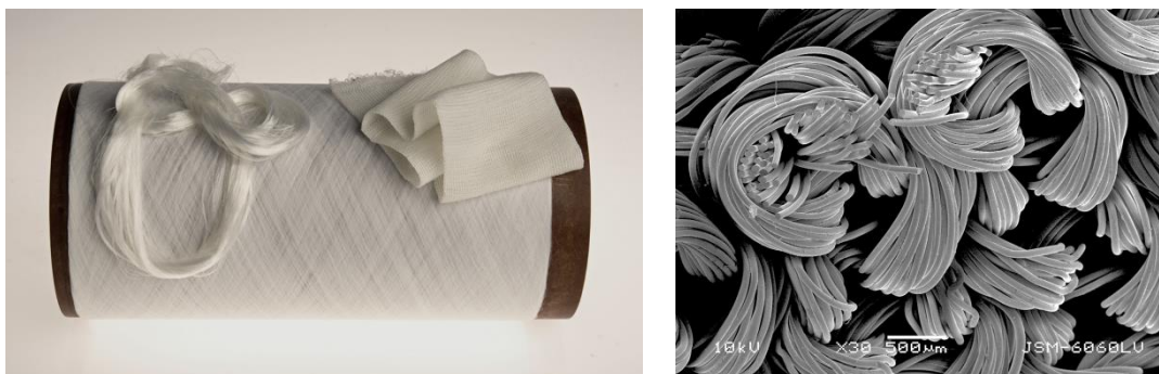
Figure 1. FR PA6 nanocomposite filament yarns and knitted fabric (left) and SEM images of the knitted fabric (right).
