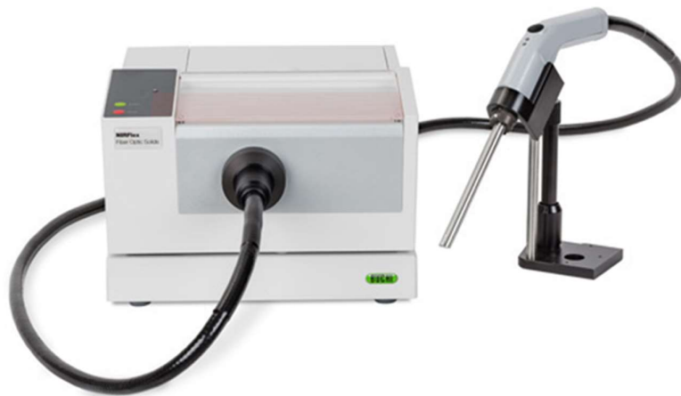
Figure 5-1. Buchi FT-NIR instrument used to collect the spectral data from the abovementioned samples.
