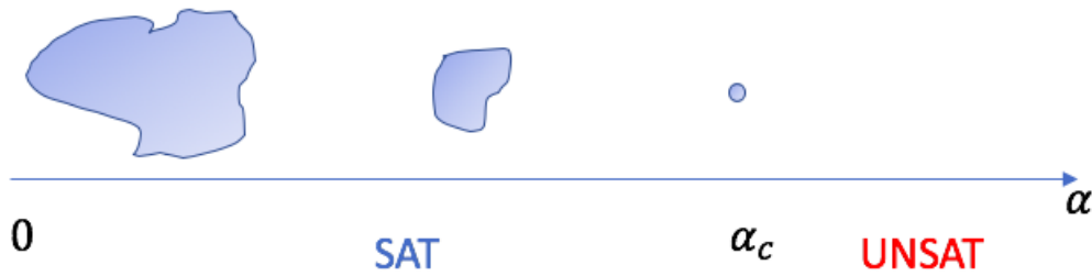
Fig. 2.4 A schematic representation on how the version space \Omega modifies as \alpha increases. It does exist a critical value \alpha_c above which the version space no longer exists and our problem is unsatisfiable.
