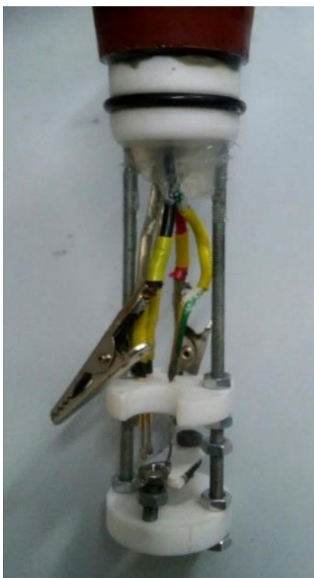
Figure 5. Support for the sensor and heater
