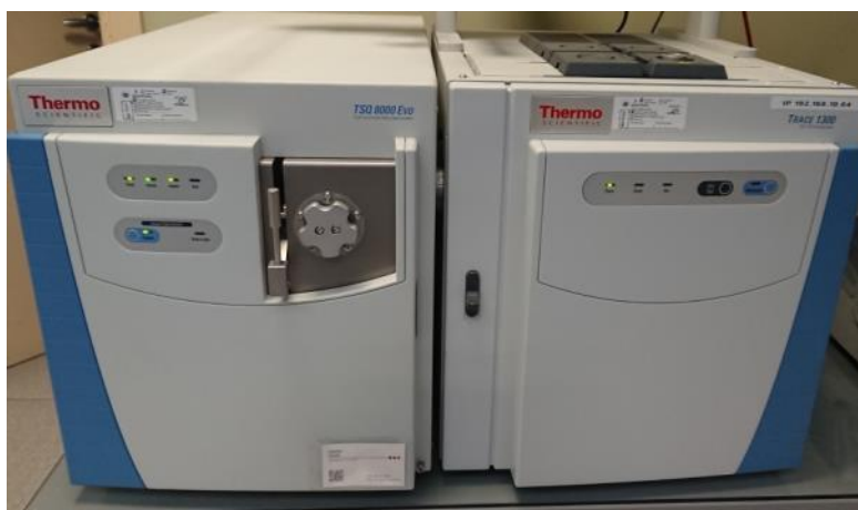
Figure 1. Thermo Scientific Trace 1300 and TSQ8000EVO triple quadrupole
