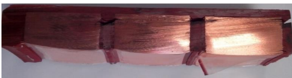
Figure 2. Cast resin transformer assembly. Epoxy resin (red part) and polyester polymer (transparent film) are clearly visible. The multilayer structure (copper-polyester alternate stacking) is evident.
