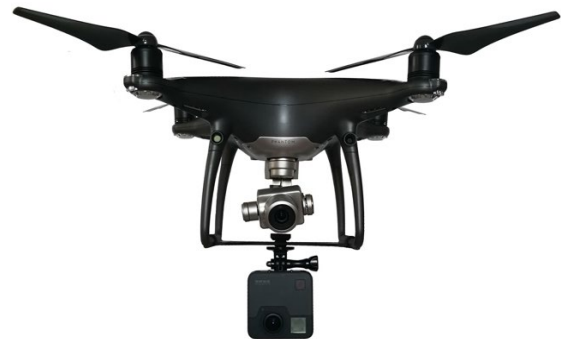
Figure 1. The UAVs/360° camera set up adopted in this research to perform a double sensor acquisition.
