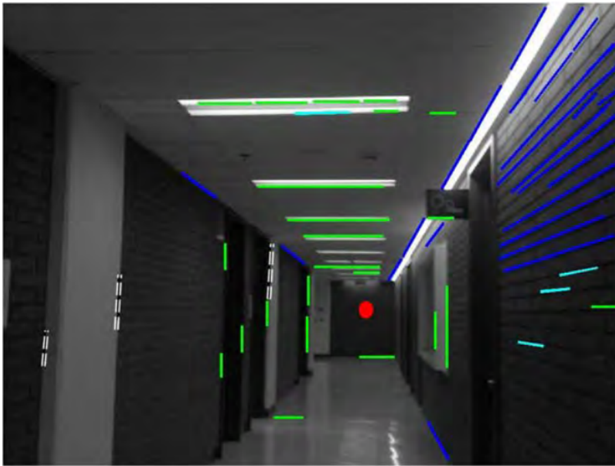
Figure 4.6: Vanishing points representation. Totally vertical or horizontal (green), vertical (white dotted), horizontal (turquoise) and along the direction of propagation (blue). Central vanishing point (red dot). Figure from [156].
