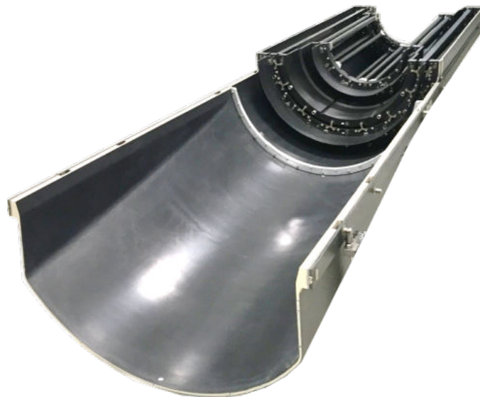
Figure 5.51: OB mechanics including the OB service barrel (in foreground).
