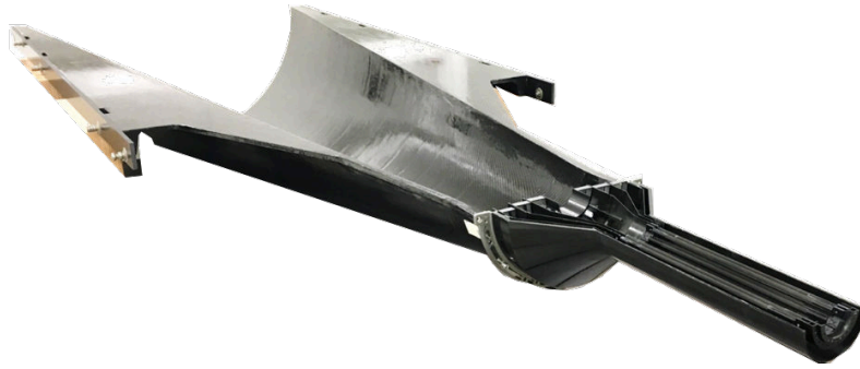
Figure 5.50: IB service and detector barrels. In particular the service barrel is shown in background while, the smaller detector barrel is shown in foreground.
