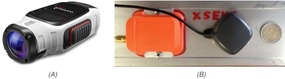
Figure 3.2. (A) Action cam Garmin VIRB® Elite; and (B) Xsens Mti-G IMU sensor with GPS antenna
