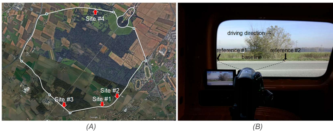
Figure 4.3. (A) Position of the control sections along the test track, and (B) picture from the trunk of the parked vehicle during recordings
