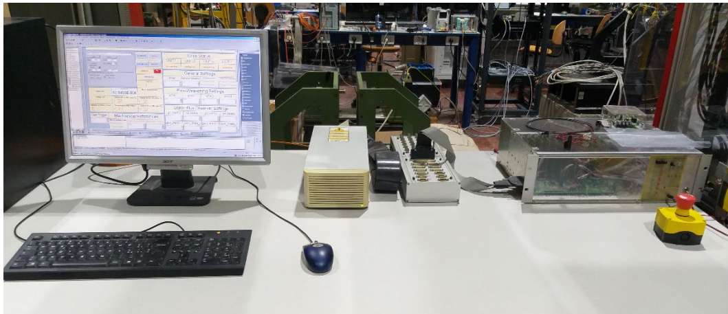
Fig. 4. 10. View of the digital controller DS1103 PPC Controller Board (left) and the power converter FPGA motherboard (right).
