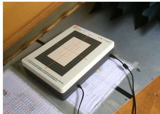
Figure 11. RFX EM-Scan inserted in the GTEM cell internal region.
