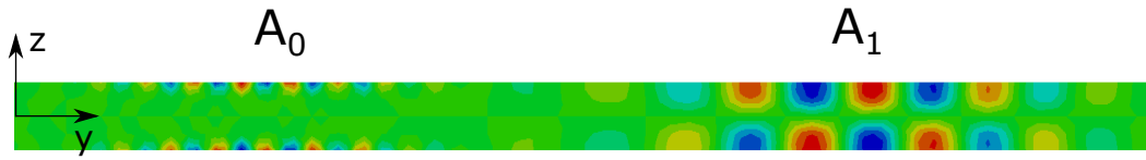
Fig. 10.12 A_0 and A_1 modes at t = 6 \times 10^{-5} for a signal burst of 1.2 MHz.
