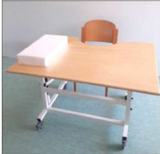
Figure 13. The patient sat on a wheelchair or on a chair depending on his/her trunk control level. The PC and the forearm support (size [cm]: 54x26x9) located on a height adjustable mobile table.
