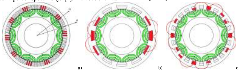
Fig 1. Cross sections of the three PM-SyR machines under analysis: a) q=3 , distributed windings; b) q=2/5 , concentrated windings; c) proposed q=4/5 solution, with mildly overlapping windings. The red areas in the slots indicate one phase. The end turns are also evidenced.
