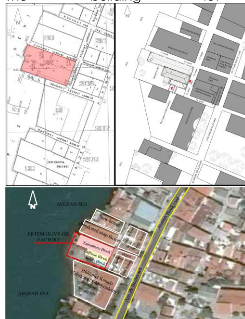
Figure 4) which is located on 14. Street, Sakarya District in Ayvalık/Balkesir-Turkey, covers an area of 1125 m 2 , of 582 m 2 which is occupied by the factory. The factory is located at the north-east part of the lot. It is composed of three blocks (See Figure 5) adjacent to each other. The main entrance to the factory is provided from 14. Street, from the middle block named as '2nd Block'. The courtyard entrance is also provided from 14. Street, through a courtyard door that is adjacent to the factory.
