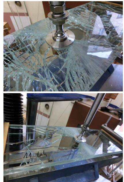
▶ Fig. 3: Non-standard connection tests of the facade glass panel performed at Klokner Institute, CTU in Prague
