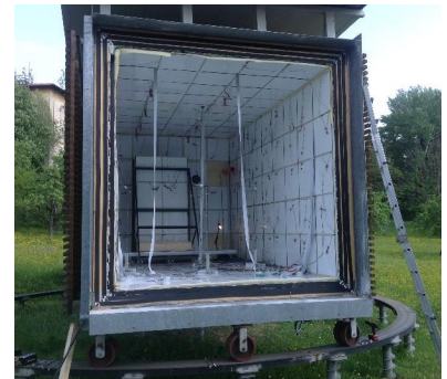
▶ Fig. 2: Overview of the Heat Flux Tiles System inside the Test room
