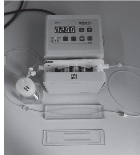
FIGURE 1: Assembled laminar flow bioreactor (LFB). Bioreactor is composed by a mixing chamber filled with a complete culture media with 5% of Dextran, a cell culture chamber, and a peristaltic pump. All the components were connected in a closed loop and put in an incubator to preserve temperature (37°C) and CO<sub>2</sub> concentration in air (5%).
