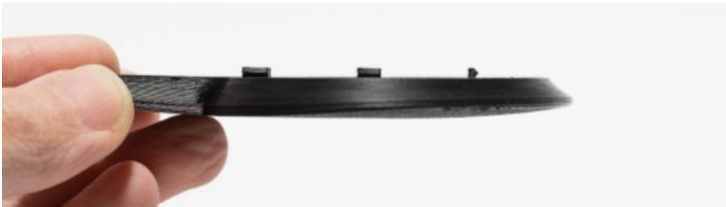
Figure 3.5 - A warped FDM part printed in ABS [31]
