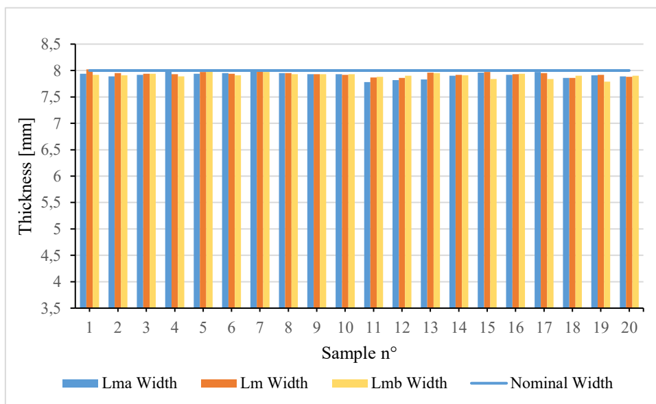
Histogram 5.3 - Lma, Lm and Lmb Width measurement performed on 20 printed Dog bone
