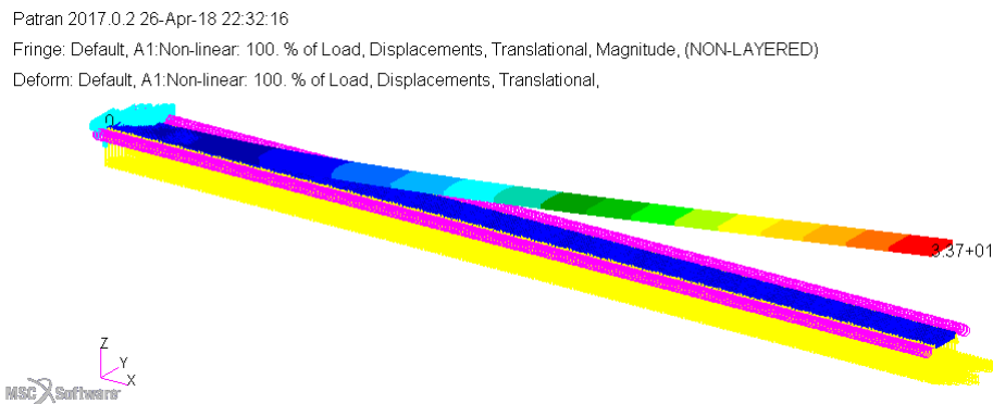
Fig. 5.24 Nonlinear static deformation for the optimized wing box with two control points ( \vartheta_1 = 0^\circ , \vartheta_2 = 10^\circ ).
