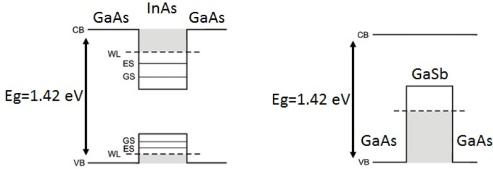
Fig. 5.5 Case studies band alignment: (a) representative of InAs/GaAs QDs. (b) representative GaSb/GaAs QDs
