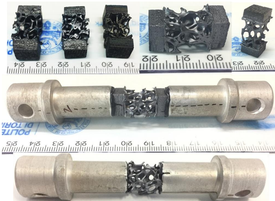
Figure 69 Sandwiches and bare SiC foam for tensile tests inside test fixtures
