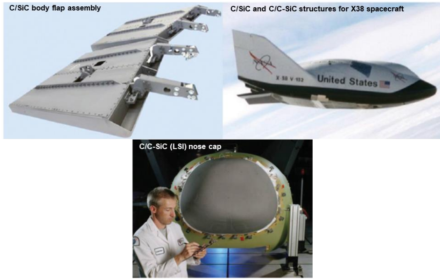
Figure 2 C/SiC and C/C-SiC application in X-38 spacecraft [1]
