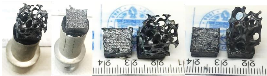
Figure 72 Typical fracture surfaces of Sandwiches from tensile tests
