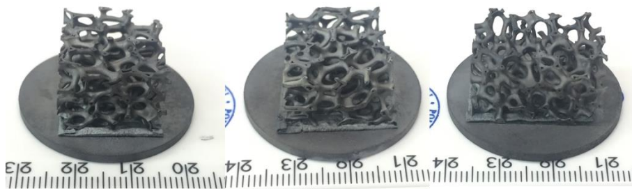
Figure 76 SiSiC disk to SiSiC foam joined in a single step by Mo-Wrap
