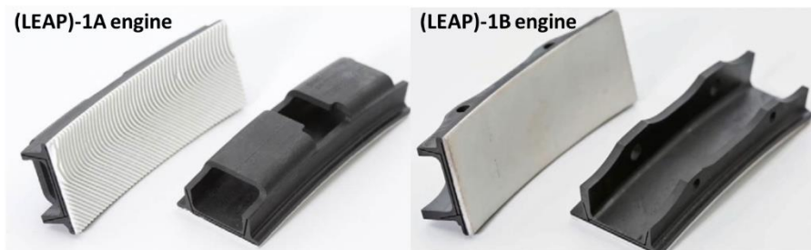
Figure 8 Prepeg melt infiltrated (prepeg-MI) ceramic matrix composite (CMC) shrouds used in LEAP engine [8]
