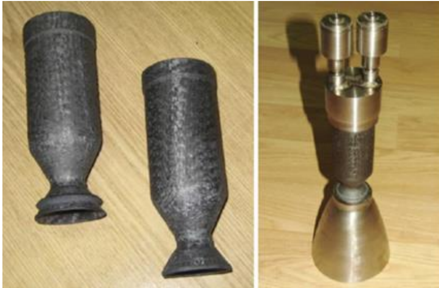
Figure 4 C/SiC (CVI) combustion chambers [1]
