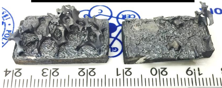
Figure 70 fractured surfaces after compression test
