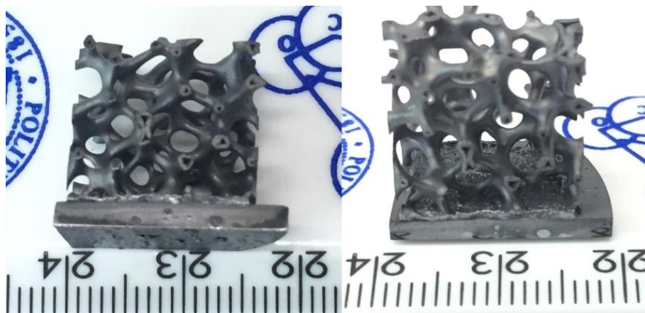
Figure 78 SiSiC disk to SiSiC foam joined by Mo-Wrap (two-step)
