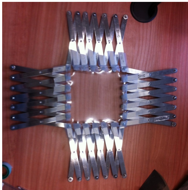
Figure 23 Squared pantograph structure
