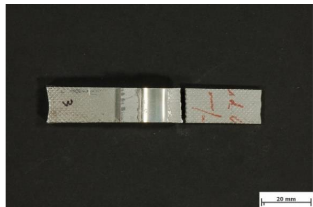
Figure 8. The tensile test result of SiC p /Al MMCs joint.
